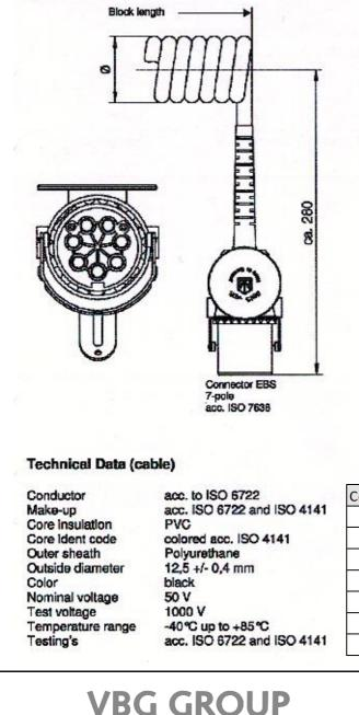
Cable PVC/PUR black  $2x4,0 + 3x1,5 + 2x1,5 mm^2$ Coll Ø 60 +-10 mmBlock length = 390 +- 50 mmWorking length:2.250 mmMax. extension length:4.000 mmRequirementsacc. ISO 4141 part 1, 2, 4TightnessIP67 and IP69K acc. DIN 40050
